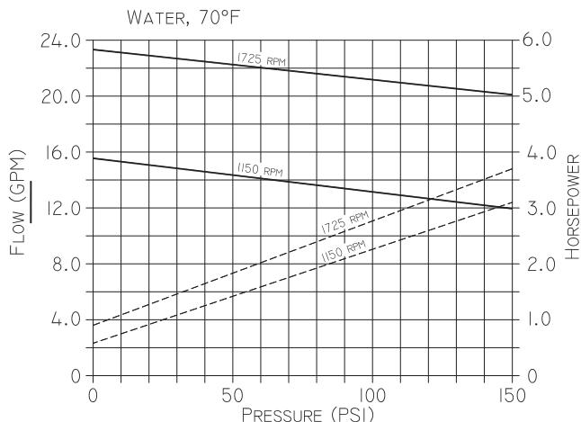
The recommended liquid temperature range is 32° to 140°F for longest pump life. If more extreme temperature conditions exist, our factory should be consulted. Freezing of water-filled pumps can cause damage and must be avoided. Oils at low temperatures are very viscous requiring a lower speed or extra power.
